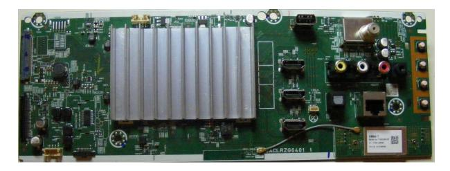
When replacing the Digital Main, the antenna cable must be removed from the defective board installed on the replacement board.
