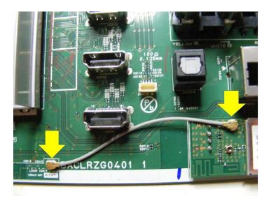
Failure to move the cable will result in the lack of range for the microphone.
