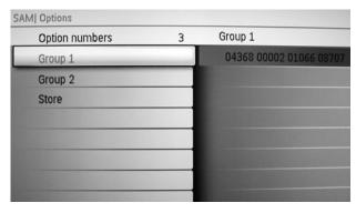
6. Cursor back to the SAM main menu and select STORE. Cursor right, then press OK to store the changes. STORE COMPLETE or a similar message should be displayed. Turn the TV off then back on to activate the changes. SSB configuration is complete.
